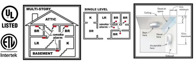
A "Listed Smoke Alarm" has been tested to ensure it meets minimum industry standards. "Listed" alarms will have either the UL or ETL mark on them.
